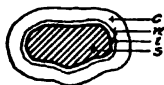
FIG. 31. — Diagram showing the relationship of the hygroscopic and capillary water films surrounding a soil particle. (s), particle; (i), zone of influence of particle; (w), outer edge of hygroscopic zone; (c), capillary film.
